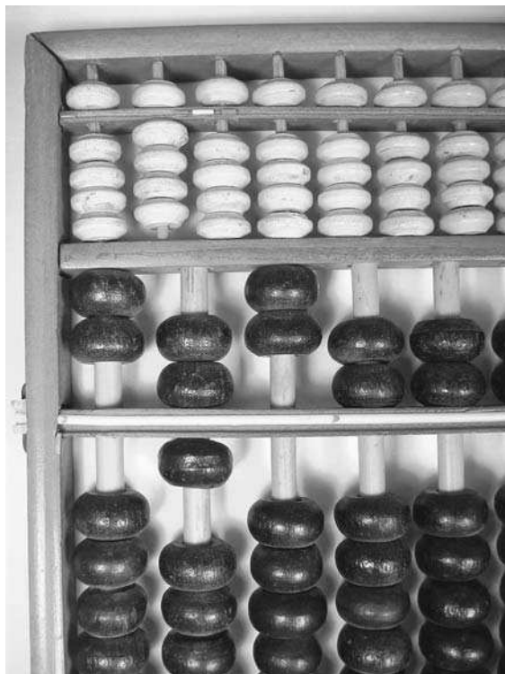
abacus A special form of the Chinese abacus (c. 1958) consisting of two abaci stacked one on top of the other. Luis Fernandes
